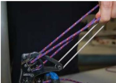
**9** Feed it through the double block from the bottom of the block and through the non-becket side. Make sure the becket is on the port side.
